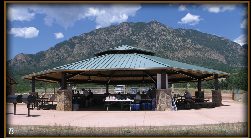
Cheyenne Mountain, Colorado Springs, CO: 58'-6" Savannah model 12" o.c. standing seam steel roof, 4:12 pitch, in Hemlock Green color. 2" x 6" cedar T&G sub-roof & cedar fascia.
