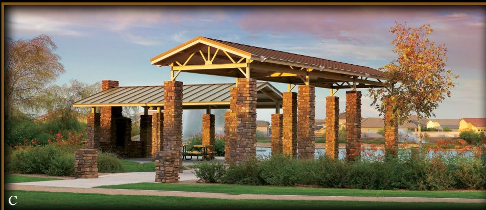
Rancho El Dorado, Maricopa, AZ: Custom 13'-8" x 46' & 20' x 32' Orlando models are centerpieces located at the entrance of a new upscale housing community. Custom masonry & faux stone surrounds underlie an I-beam frame and a Marine Green standing seam steel roof with tubular steel fascia.
