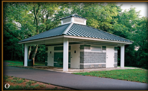
Knoxville, TN: 22' 6" x 22' 6" custom covers a site-built block restroom. Cool Weathered Copper standing seam roof.
